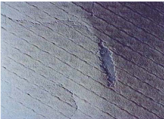
scaled membrane Surface With Imprints from the feed spacer
