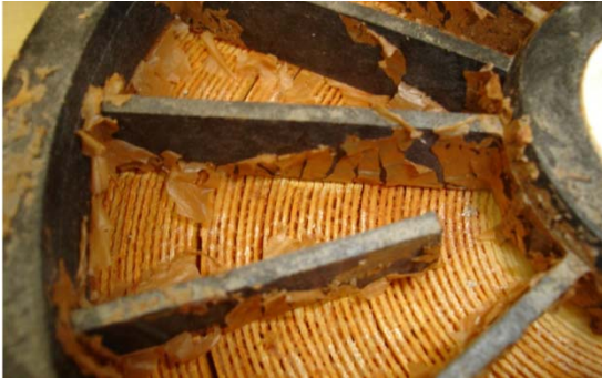
Heavy Metal Fouling in lead (1 st ) element
