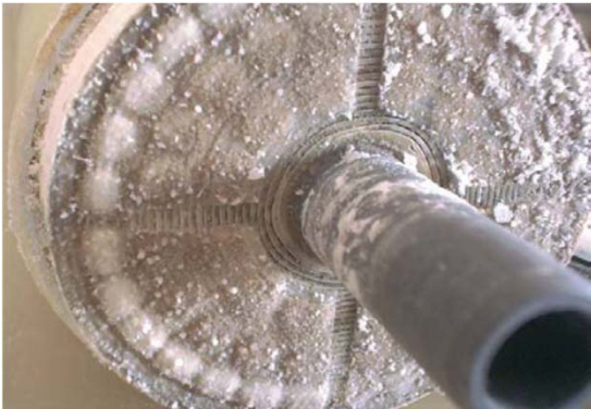
Calcium Sulphate scaling last stage element
