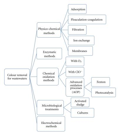
FIGURE 5: Methods for textile wastewater color removal.
