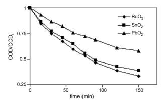
Fig. 6. The effect anode material on rate of degradation; supporting electrolyte concentration  $0.58 \text{ g} \text{ l}^{-1}$ ; current density 3 A/dm<sup>2</sup>; pH 7.
