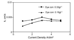
Fig. 8. Variation of transfer coefficient with current density; supporting electrolyte concentration  $0.58 \text{ g} \text{ l}^{-1}$ ; pH 7.
