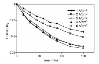
Fig. 3. Influence of the current density on  $COD/COD_i$  with electrolysis time. Dye initial concentration  $0.33 \text{ g} \text{ l}^{-1}(COD_i: 350 \text{ mg} \text{ l}^{-1})$ ; supporting electrolyte concentration  $0.58 \text{ g} \text{ l}^{-1}$ ; pH 7.
