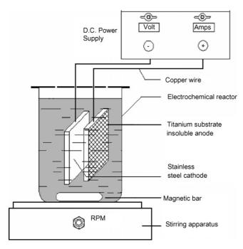
Fig. 2. The schematic diagram of experimental setup.
