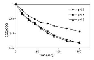
Fig. 4. The effect of pH on pollutant degradation; dye initial concentration  $0.33 \text{ g} \text{ l}^{-1}$ ; supporting electrolyte concentration  $0.58 \text{ g} \text{ l}^{-1}$ ; current density  $3 \text{ A/dm}^2$ .
