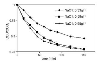
Fig. 5. The effect of supporting electrolyte concentration on pollutant degradation. Initial dye concentration  $0.33 \text{ g} \text{ l}^{-1}$ ; current density  $3 \text{ A/dm}^2$ .
