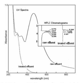
Fig. 9. UV-vis spectra and HPLC chromatogram of raw and electrochemically treated Acid Brown 14 dye wastewater.
