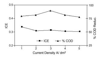
Fig. 7. Variation of ICE along with COD reduction with current density; supporting electrolyte concentration  $0.58 \text{ g} \text{ l}^{-1}$ ; current density 3 A/dm<sup>2</sup>; pH 7.
